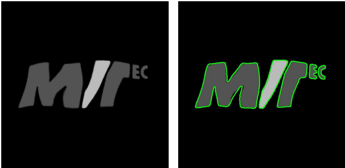
Figure 3.41: (left) search image; (right) search image overlaid by deformed contours.
