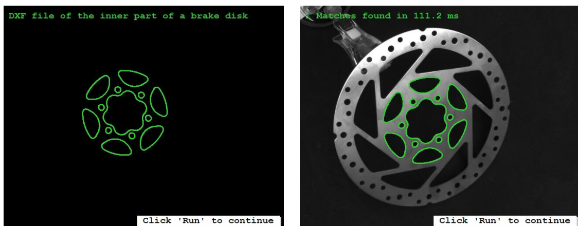
Figure 2.10: (left) synthetic XLD model accessed from a DXF model; (right) model found in a search image.
