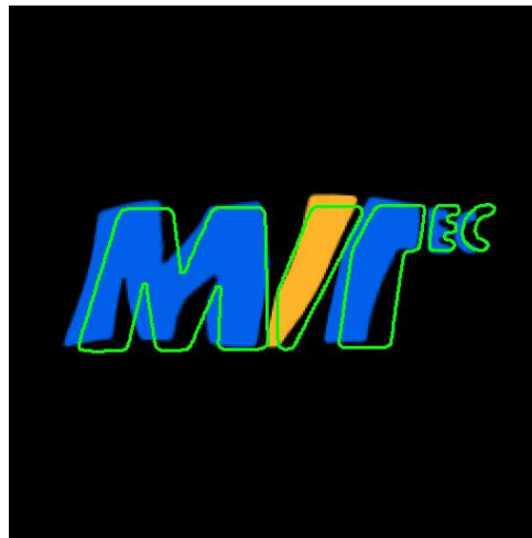
Figure 1.6: Object consisting of two components that move relative to each other.
