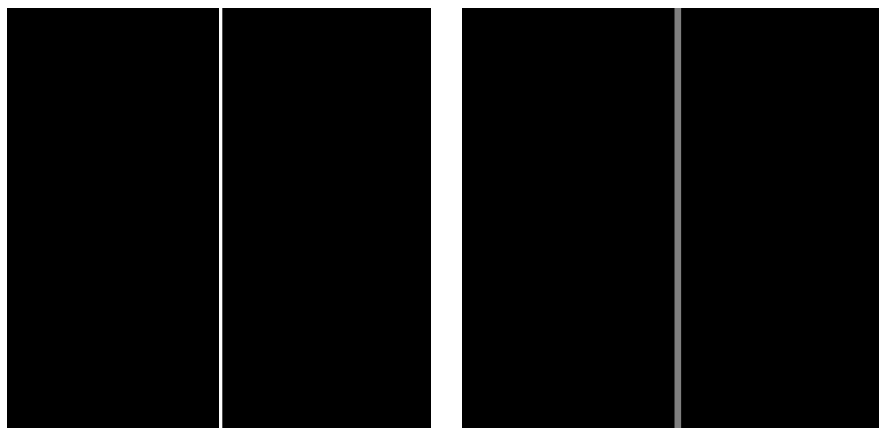
Figure 2.12: In the pyramid, a (left) one pixel wide high contrast line blurs to a (right) broader line with a lower contrast.
