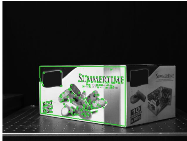
Figure 1.4: 3D object: unique parts of the object lie in a plane and can be described by clearly visible contours.
