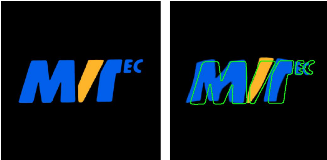
Figure 3.36: (left) “MVTec” logo used for the model creation; (right) deformed logo instance overlaid by the model contours.
