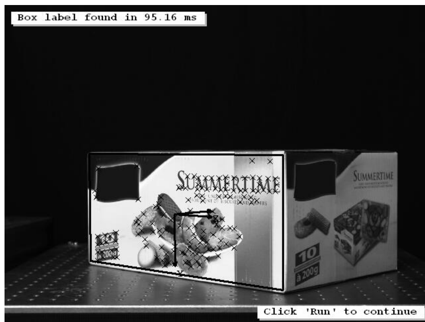
Figure 3.46: 3D pose of cookie box label obtained by calibrated descriptor-based matching.
