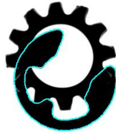
Figure 1.8: Occlusions can be handled by shape-based matching.
